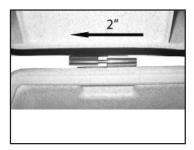
In severely confined spaces, removing the mounting knobs and sliding the toilet away from the mounting location may be a more desirable method of servicing the unit.
