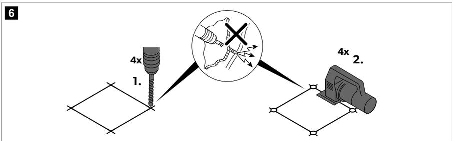
5. Carefully cut out the opening on the roof using a keyhole saw or a similar tool (**B**).
