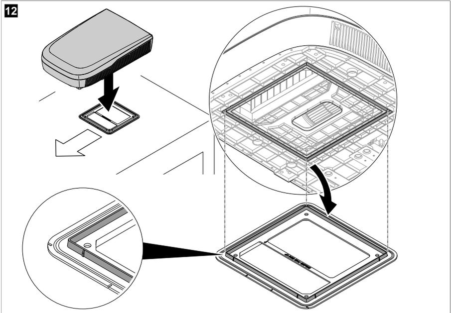
21. Lift the roof top unit onto the roof of the vehicle. Observe the direction of travel.
