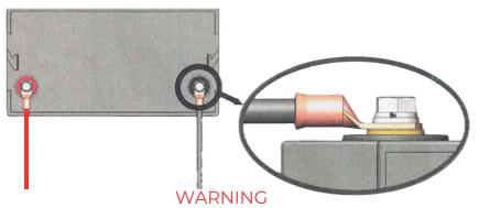
Reversing polarity could cause damage to load or battery
