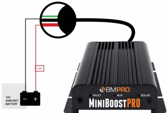
Figure 6: Selecting the 12V AGM/ WET Battery
