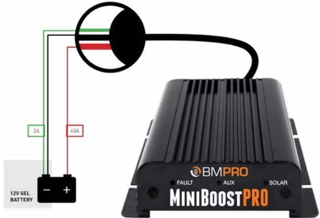
Figure 5: Selecting the 12V Gel Battery
