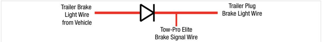
This prevents the back feeding of 12V into the vehicle when the Tow-Pro is manually activated whilst illuminating the trailer brake lights.
