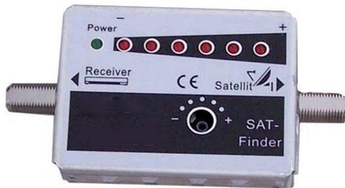
The Sat-Finder is a simple instrument for setting and building the satellite antenna. The satellite finder is used to adjust the satellite dish and LNB set up the position.
