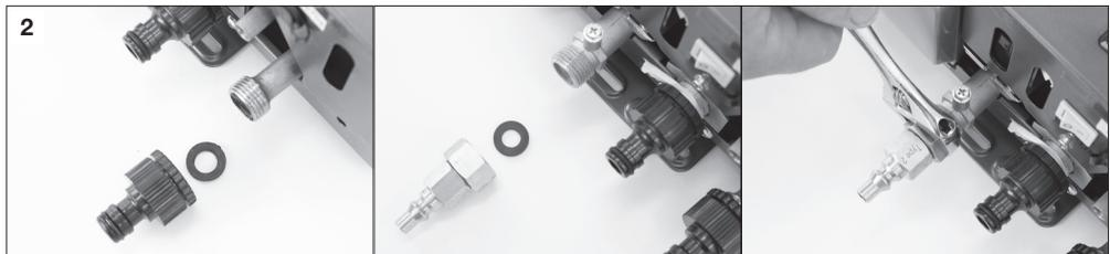
2. Attach the 1 x Gas and 2 x Water adapters to the inlet connections on the base of the unit. Use the supplied Thread Tape prior to attaching the adapters and ensure all are fitted with the Black Rubber "O" Rings. The Male GAS Adapter must be tightened with a spanner – DO NOT FINGER TIGHTEN.
