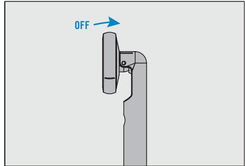
**Step 2.** Remove pump safety cap and push on/off switch to start the pump.
