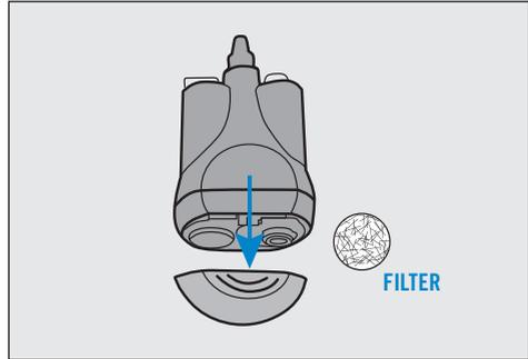
**Step 2.** Clean the filter and filter cover using clean fresh water only.
