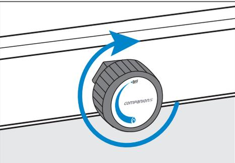
Press the gas control and turn the gas controls full clockwise to the OFF position.
