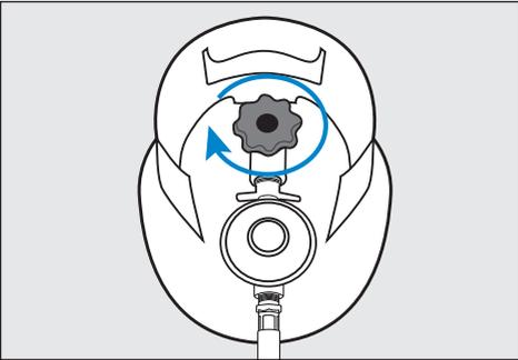
With the flame still operating, turn the valve on the gas cylinder in a clockwise direction until it is OFF. Allow the flame to burn down then extinguish once all remaining gas in the hose has been used.
