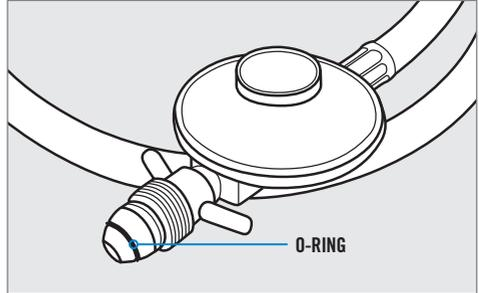
Figure 1: O-RING seal on the POL regulator.
