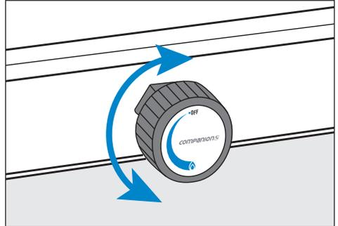
**Note:** When operating the appliance in windy conditions it is important to regularly check the burner to ensure that the flame has not been extinguished. If so turn the gas control off, allow residual gas to disperse. Relocate the appliance to a more sheltered position before attempting to reignite the burner.
