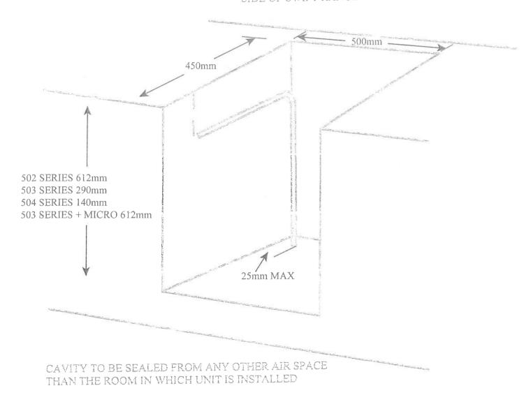
ATTENTION: The base of the appliance must be supported by either a full flat base level with the bottom edge of the cavity opening or a support bar across the rear of cavity below where the back frame of the cooker will sit.
